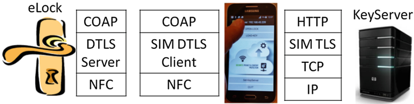
Fig. 13. COAP electronic lock prototype.
